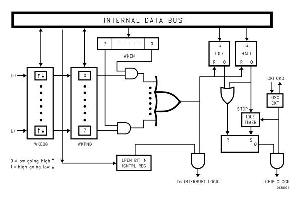
FIGURE 21. Multi-Input Wake-Up Logic
