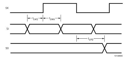
FIGURE 1. MICROWIRE/PLUS Timing
