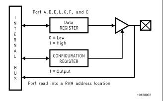
FIGURE 4. I/O Port Configurations — Output Mode
