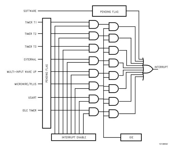
FIGURE 26. Interrupt Block Diagram
