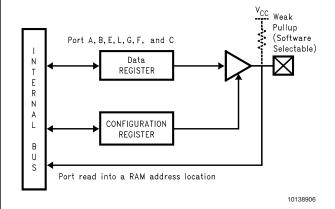
FIGURE 3. I/O Port Configurations
