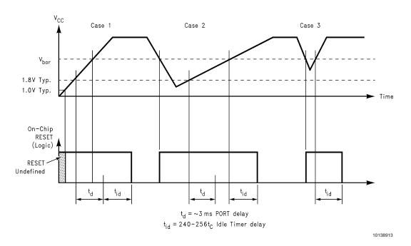
FIGURE 10. Brownout Reset Operation
