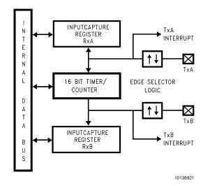
FIGURE 18. Timer in Input Capture Mode
