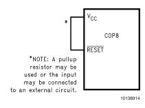
FIGURE 11. Reset Circuit Using Power-On Reset
