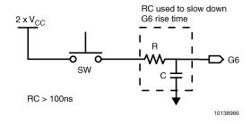
FIGURE 14. Circuit Diagram for Implementing the 2 x
