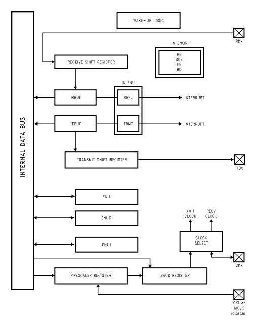
FIGURE 22. USART Block Diagram
