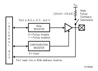
FIGURE 5. I/O Port Configurations — Input Mode
