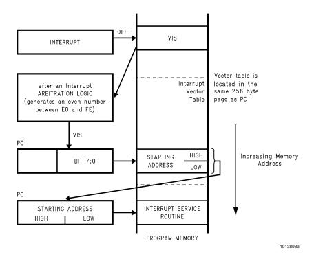
FIGURE 27. VIS Operation
