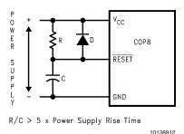
FIGURE 9. Reset Circuit Using External Reset
