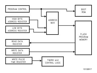
FIGURE 13. Block Diagram of ISP
