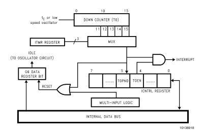
FIGURE 15. Functional Block Diagram for Idle Timer T0
