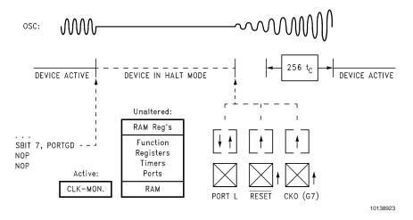
FIGURE 20. Wake-up from HALT
